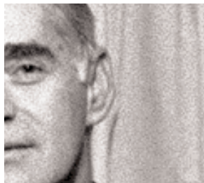
Detail of a print showing the cracked pattern of a reticulated negative.
