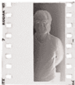
On many cameras, the shutter won’t sync with the flash when the shutter is set at too fast a speed. Here, the shutter speed was 1/500, causing only half the film to be fully exposed.
