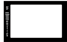
LED display: for camera's with aperture-priority, when the f-stop is set the corresponding shutter speed is displayed in the scale on the left.
